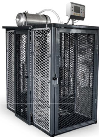
Safety inflation cage for large tyres. The cage is incl. a PCI 1000 high-flow computer inflator for 12 Bar. EM SAFE is fitted with a door on the side and an Omega-Jet system (22,5"), roll-out system and emergency emptying system with a 10-metre cable and a door switch. EM SAFE can also be purchased only as a cage without any additional equipment.
