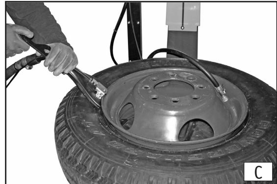
**6-** The air jet develops a series of forces inside the tyre which allow the bead to be inserted in the rim.
