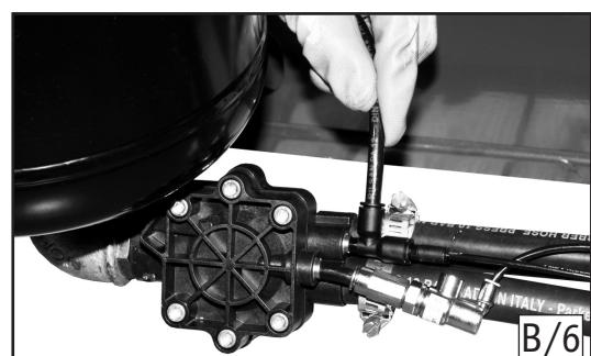
**9-** Remove the plastic cap (**1, Fig. B/3**) from the rear of the machine body, then lead the hose just fitted out of the hole opened.
