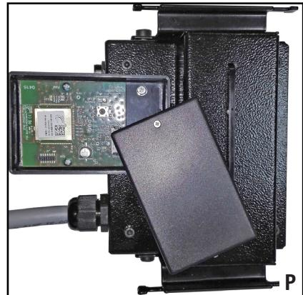
1) Remove the cover of the transmitter radio module by unscrewing the screw (fig. P) to access the electronic board.
