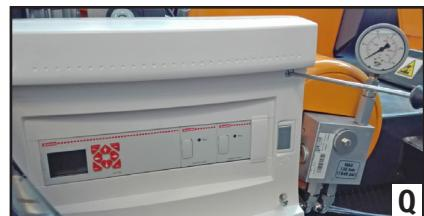
2) Remove the receiver cover by unscrewing the 4 screws (fig. Q) to access the electronic board (fig. R).
