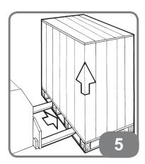
Before installation, the machine must be transported inside its original packing, making sure the product is maintained in the position indicated on the outer packing. The machine can be moved by placing the packages on a wheeled trolley or inserting the forks of a fork lift in the relative openings in the pallet (Fig.5).
