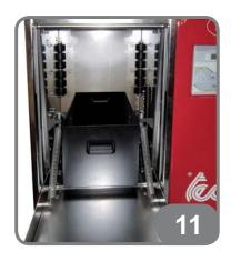
Once the collection basket has been correctly placed inside the washing camber the two openings on the sidewalls of the collection basket shall face each one the washing nozzle mounted on the sidewalls of the washing chamber.
