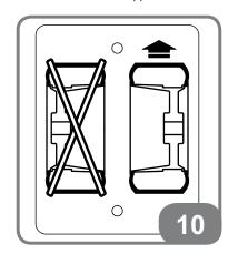
The washing and drying systems on either side of the washing chamber are optimized so that optimal washing and drying effect is achieved by placing the outer side of the wheel facing right (Fig.10). Placing the wheel inside the washing chamber with the outer side facing left will lead to reduced effectiveness of both the washing system and the drying system.
