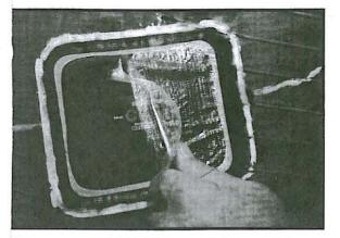
Next, remove the clear poly from the Centech repair unit. If the repair unit is to be cured in a rimless retread chamber, apply #738 Security Coat before curing. If curing in a section mold or a retread system that has a curing tube or inner envelope, apply #738 Security Coat after cure.
