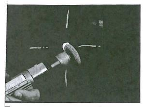
Continuing with the same rasp or inner liner wheel, overbuff around the exterior of the skive by at least 1"or 25mm.
