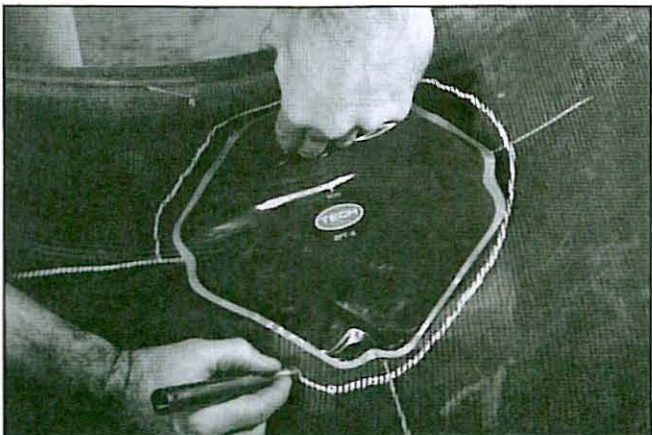
42 Using the index lines, center the previously determined repair unit over the injury and draw a perimeter approximately 1" (25mm) around the circumference of the repair unit. This is to be used as a guide for mechanical buffing.
