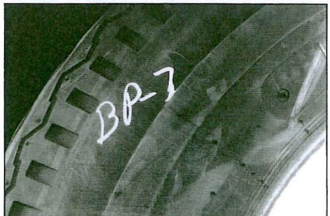
19 Write the size of repair unit needed on the outside of the tire.
