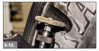
Use a medium grit buffing rasp (FCBZ21470 or RH300) or encapsulated brush (S890 or S897) on a low RPM buffer to buff the skived rubber above the steel body cables. The skive should be angled to 60° and buffed to a #2 or #3 buffed texture.
