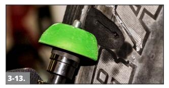
Using a fine grit buffing rasp (RH107 or FCRT3CT50) on a low RPM buffer, buff the outside surface of the tire 1" (25mm) wider than the cavity being prepared. Buffing this area to a #1 or #2 surface will promote proper bonding of the overflow rubber as the repair cures.
