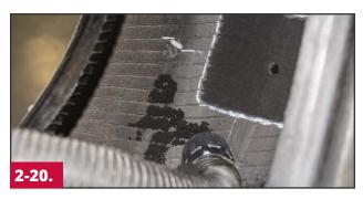
Vacuum all of the buffing dust from the tire. Do not touch the buffed surface with the vacuum as this could lead to contamination.
