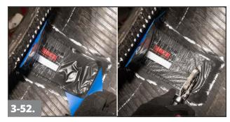
Remove the poly from under the repair unit and continue stitching from the center toward the edges of the repair unit.
