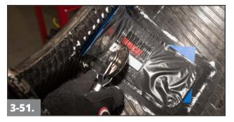
Press down the center of the repair unit with your thumb or the side of your hand. Begin stitching the repair unit from the center out, using firm pressure. Stitch out to the folded poly.
