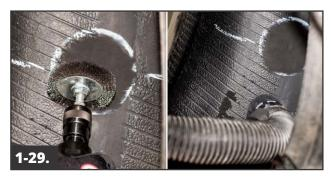
Clean the buffed surface with a soft wire brush on a low RPM air buffer, working from the right side of the buffed area to the left. Repeat until all buffing dust is removed. Vacuum all buffing dust from the tire. Do not touch the buffed surface with the vacuum, as this will lead to contamination.
