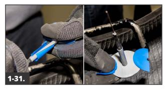
Remove the poly from the stem by pulling on the tapered portion of the stem and twisting until it releases. Remove and reposition the poly on the cap to prevent contamination of the cushion gum and to allow for easier removal of trapped air from under the repair during installation.
