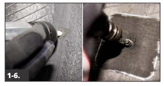
If necessary, use a pencil shaped aluminum oxide stone on a high speed grinder (20,000 RPM min.) to remove any remaining loose steel cables in the injury channel. Remove any scorched or burnt rubber using skive brush on a low speed buffer.
