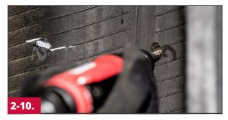
Remove any scorched or burned rubber using a skive brush on a low speed buffer.
