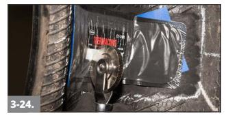
Press down the center of the repair unit. Begin stitching the repair unit from the center outward using firm pressure. Stitch the repair unit out to the folded poly.
