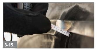
If necessary based on the curing equipment being utilized, measure the thickness of the tire in the repair area so that curing time can be calculated. Refer to page 34 for more information on calculating cure times.
