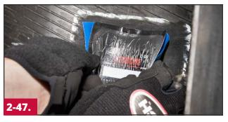
Fold and position the repair unit so that the repair unit's bead arrows are pointed toward the tire's beads. Center the repair unit over the injury and place the center of the repair unit against the inner liner. Release the repair unit and check that the repair unit is properly aligned and centered. If the repair unit is not centered, and/or straight, lift and reposition the repair unit.
