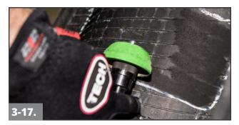
Using a fine grit buffing rasp on a low RPM buffer (5,000 RPM max.), buff the marked area on the inner liner to a #1 or #2 buffed texture. To prevent contamination of the buffed surface, avoid buffing into the crayon marks.
