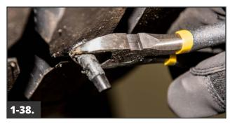
Cut off the excess stem 1/8" (3mm) above the tire's outer surface. If the tread has been buffed off, use rough grit buffing wheel on a low RPM buffer and buff the stem flush with the tire's buffed surface.
