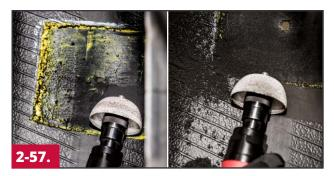
Once the sealant material has been completely removed from the casing, buff the exposed area of the casing with a fine grit buffing wheel (RH107, FCRT3CR50 or equivalent) on a low RPM buffer to a #1 or #2 buffed texture. Also, buff a 1-1/2" (40mm) area on the inner liner on all sides of the exposed area with the buffing wheel rotating inward toward the cut edge of the inner liner.
