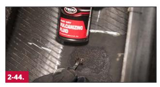
Apply a thin, even coat of cement by stippling the cement onto the inner liner. Use Chemical Vulcanizing Fluid #760 or Heavy Duty Blue Vulcanizing Fluid #775 for cold, or chemical cure applications. Allow the cement to dry thoroughly. **Note: Dry time for #760 is 3 – 5 minutes, #775 is 5 – 8 minutes. Allow additional drying time in cold and/or humid conditions.**
