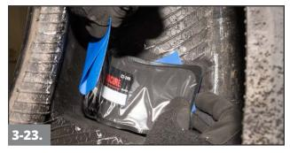
Fold the repair unit, then position the repair unit over the buffed surface, aligning the bead arrows toward the tire's beads. Place the repair unit over the injury and check the alignment. If the repair unit is not straight and/or properly positioned within the buffed surface, lift the repair unit and reposition.
