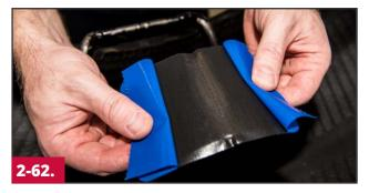
Break the perforation on the back of the repair unit and expose the center of the repair, leaving the protective poly on both ends.
