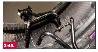
Once the cement is dry, release the spreader so that the tire is in a relaxed position prior to installing the repair unit. This will reduce the risk of bridging the repair unit.
