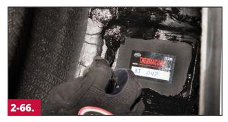
Apply Butyl Liner Repair Sealer #739 or Security Coat #738 to the edge of the repair unit, Vul-Gum and the over buffed area on the inner liner.
