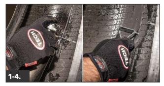
Pre-clean the inner liner with TECH Rub-O-Matic #704 or 704A and a Scraper #933 2 to 3 times to remove contaminants from the inner liner.
