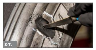
Using a skive knife, cut along the outer edge of the damaged cables. Leave as much rubber as possible in the tire.
