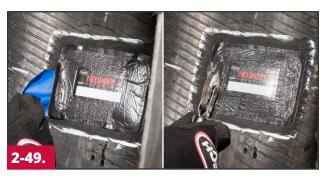
Remove the poly from under the repair unit and continue stitching from the center toward the edges of the repair unit.
