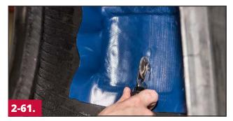
Place the cushion gum over the buffed area and stich the cushion gum from the center out. Be sure not to trap air in the transition area between the casing and the inner liner.
