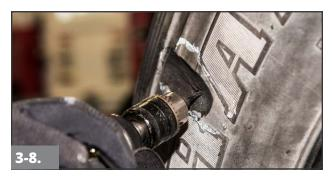
Using the appropriate carbide burr on a high RPM buffer (20,000 RPM min.), remove all damaged steel at a 90° angle to the tire. Steel cables must be cut back to solid rubber.
