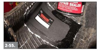
Apply Butyl Liner Repair Sealer #739 or Security Coat #738 to the edge of the repair unit as well as to any buffed surface not covered by the repair unit. Allow the tire to sit for 24 hours before returning to service.
