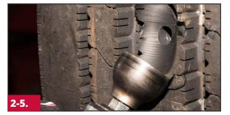
Use a knife or rotary gouge on a low RPM tool (5,000 RPM max.) to remove any loose or damaged rubber. Be careful to avoid contacting the steel cables as this could lead to additional damage.
