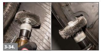
Clean the buffed area on both inside and outside of the tire using a soft wire brush on a low RPM buffer. Remove the buffing dust by lightly brushing the buffed area from the right side to the left. Repeat the process a minimum of 2 - 3times to ensure that all buffing dust is removed.
