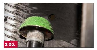
Using a fine grit buffing wheel (#RH107 or #FCRT3CR50 or equivalent) on a low RPM buffer (5,000 RPM Max.), buff an area approximately 1  $\frac{12}{2}$ " (40mm) in all directions around the injury.
