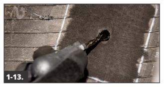
Using a fluted or spiral cement tool, apply black TemVulc cement into the injury.
