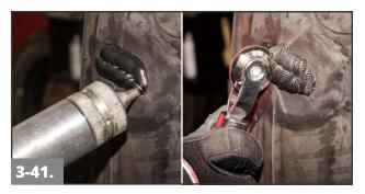
Finish filling the cavity with rope rubber until the rubber is built up 1/8" (3mm) above the tire's surface. Stitch the rubber using firm pressure to remove trapped air. The tire is now ready for curing.
