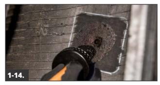
Apply a thin, even coat of TemVulc cement to the buffed surface. Allow the cement to dry for 8-10 minutes. In cold and/or humid conditions, additional drying time will be needed.
