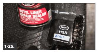
Apply Butyl Liner Repair Sealer #739 to the edge of the repair unit and to the overbuffed surface on the inner liner to retain proper air retention.
