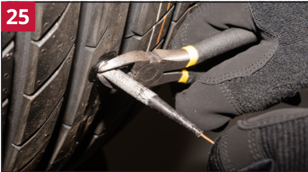
With the stem relaxed, cut off the excess 1/8" (3mm) above the tread surface.
