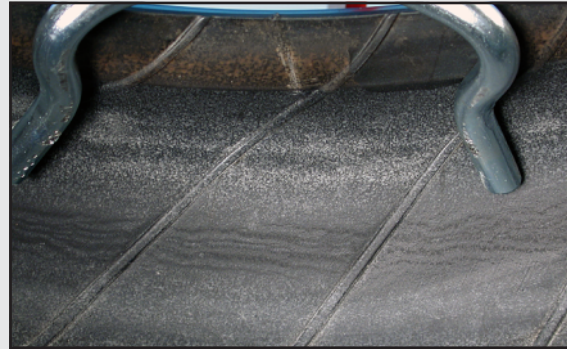
Inner Liner Cracking
