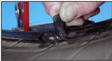
7. Deformed bead, exposed fabric or steel
