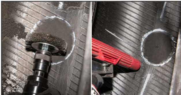
12. Use a soft wire brush on a low speed buffer to remove buffing dust and debris from the buffed area. Avoid applying excessive pressure, as this could remove texture and reduce adhesion of the repair unit to the tire. Remove the debris from the tire using a vacuum.
