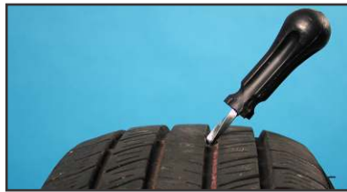
8. If injury angle exceeds 35 degrees, a 2-piece repair must be used.
