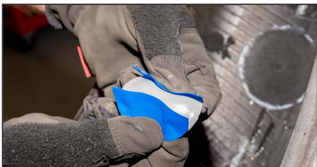
14. Bend the repair back and push up on the edges of the repair with your fingers to break the perforation on the protective poly on the back of the repair. Partially remove the poly, exposing the middle portion of the repair.
