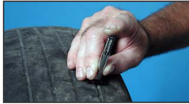
5. Excessive tread wear
