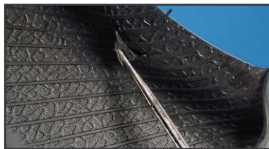
10. Tire damage from impacts
