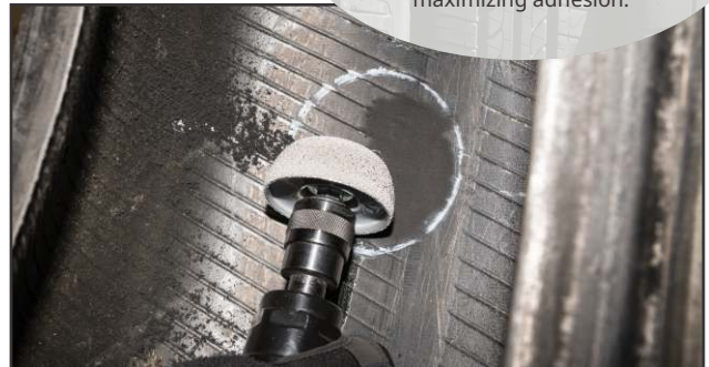
11. Using a low speed buffer (maximum 5,000 rpm) and an appropriate inner liner wheel, buff the stem flush to the inner liner. Buff the entire outlined area on the inner liner to a #1 or #2 texture.
