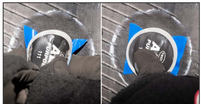
15. Relax the beads of the tire. Center the repair unit over the filled injury. Press down the center of the repair unit with your thumb. (If the repair is a Centech or BP repair unit, be sure to align the bead arrows with the beads of the tire.)
